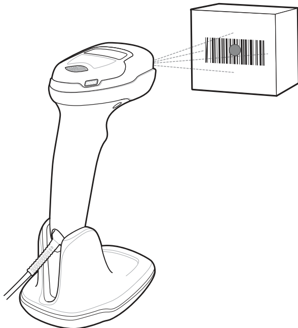
Figure 2-8 Scanning with the DS4308P
